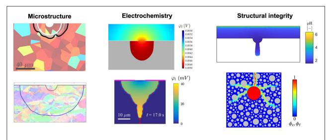
**Figure 5.** Phase-field modeling opening new horizons in corrosion research. Examples of applications: unraveling the role of microstructural anisotropy, <sup>22,23</sup> resolving the electrochemistry–corrosion interplay, <sup>10,15</sup> and predicting corrosion-induced cracking. <sup>24,49</sup>
