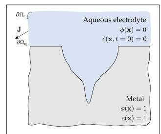
**Figure 2.** A diffusion-phase-field description of the evolution of a corroding metal assuming no mechanical straining and neglecting the influence of electric and electrochemical fields.
