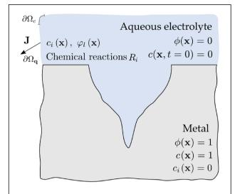
**Figure 4.** A coupled electrochemical diffusion-phase-field description of the evolution of a corroding metal assuming no mechanical straining.
