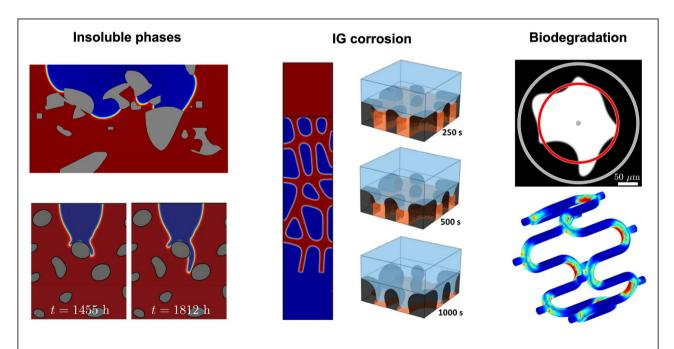
**Figure 6.** Phase-field modeling opening new horizons in corrosion research. Examples of applications: shedding light on the interplay between corrosion and secondary phases, <sup>6,7</sup> understanding the preferential path of corrosion along grain boundaries (intergranular corrosion [IG]), <sup>55</sup> and predicting "*in vivo*" the biodegradation of Mg alloys. <sup>26</sup>
