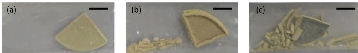
Fig. 8. Photographs of selected specimens: (a) 10 h at 700 °C, (b) 10 h at 850 °C and (c) 1 h at 1050 °C. Photographs of specimens oxidised at 850 °C and 1050°, show oxide scale that spalled off from the specimen during handling, next to the specimens. The scale bar is 5 mm. (For interpretation of the references to colour in this figure legend, the reader is referred to the web version of this article.)
